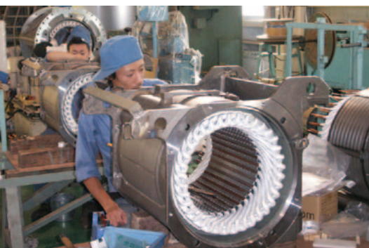
Inserting the coil into the drum, the final stage of motor coil production.
