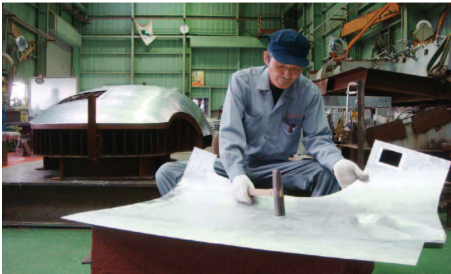
Hammering an aluminum sheet into shape.
